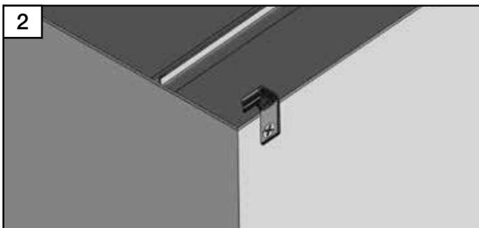
2. Position the clip on the outside of the rim joist securing it with a single screw inserted perpendicular to the joist. After positioning the last deck board in place, secure it by angling a screw through the clip and into the board at a 30°- 45° angle. Be careful to make sure the screw inserts fully and pulls the board down (3). Space no more than 12" (30 cm) apart.
